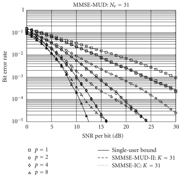
FIGURE 9: BER versus average SNR per bit performance for the MC DS-CDMA using Gold-sequences and having a  $T$  domain spreading factor of  $N_e = 31$ , when communicating over frequency-selective Rayleigh fading channels.
