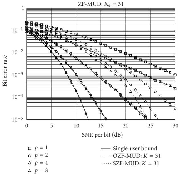
FIGURE 5: BER versus average SNR per bit performance for the MC DS-CDMA using Gold-sequences and having a  $T$  domain spreading factor of  $N_e = 31$ , when communicating over frequency-selective Rayleigh fading channels.
