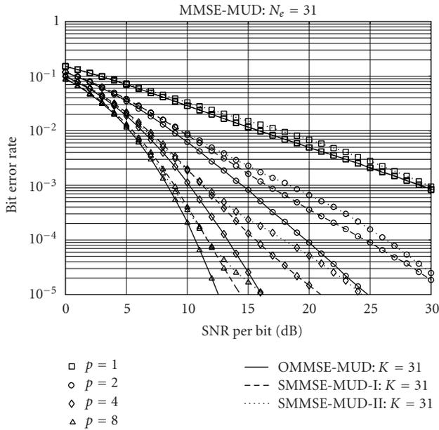
FIGURE 8: BER versus average SNR per bit performance for the MC DS-CDMA using Gold-sequences and having a  $T$  domain spreading factor of  $N_e = 31$ , when communicating over frequency-selective Rayleigh fading channels.
