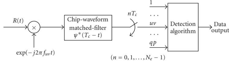
FIGURE 2: The receiver block diagram of the MC DS-CDMA systems using time-limited chip waveforms.
