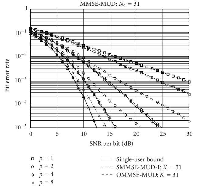
FIGURE 7: BER versus average SNR per bit performance for the MC DS-CDMA using Gold-sequences and having a  $T$  domain spreading factor of  $N_e = 31$ , when communicating over frequency-selective Rayleigh fading channels.
