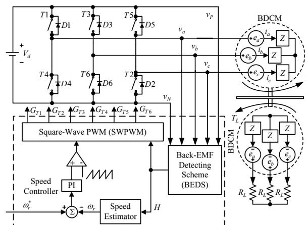
Fig. 1. sensorless BDCM control with back-EMF detecting scheme.
