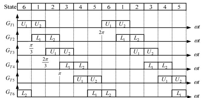
Fig. 2. Type definition of gate signals of six-step SWPWM.
