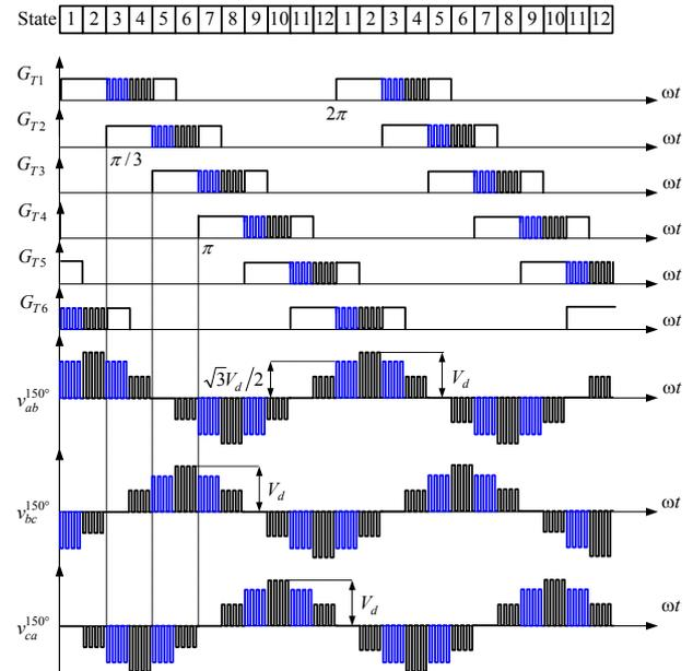
Fig. 6. Illustrated waveforms for twelve-step SWPWM type-00110\_00110.
