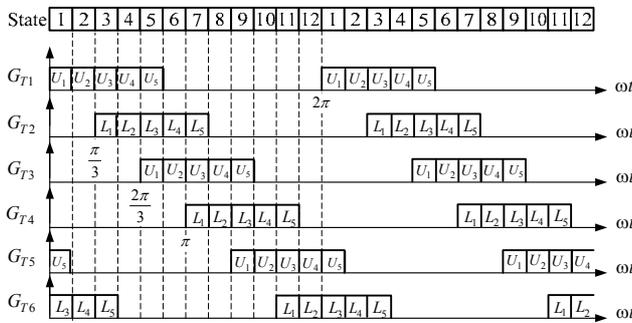
Fig. 5. Type definition of gate signals for twelve-step SWPWM.
