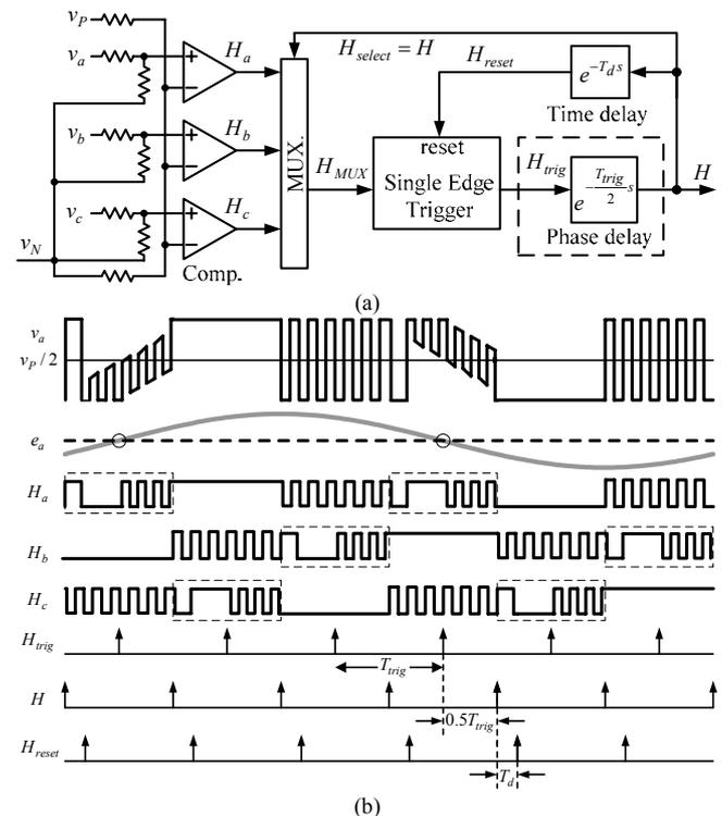
Fig. 4. (a) comparator-based BEDS for type 01\_01; and (b) its illustrated waveforms.
