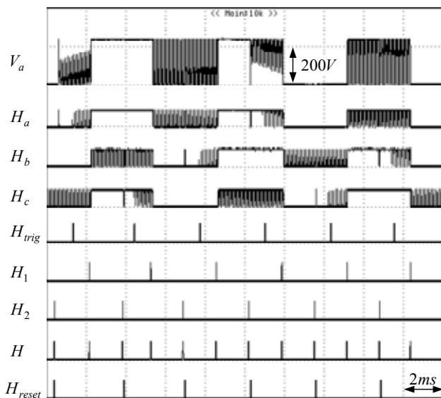
Fig. 10. Experimental waveforms for twelve-step SWPWM type 00110\_00110.
