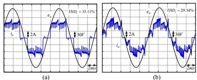
Fig. 9. Simulated waveforms:(a) six-step SWPWM type 01\_01; (b) twelve-step SWPWM type 00110\_00110.
