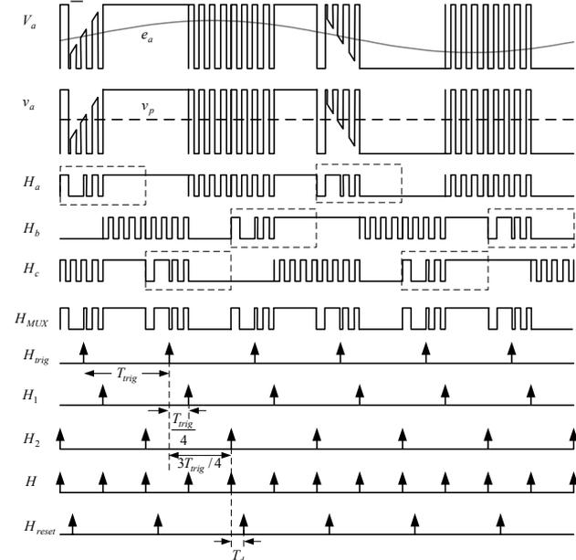
Fig. 7. Illustrated waveforms of the proposed twelve-step BEDS.
