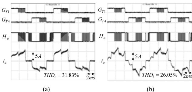
Fig. 11. Some experimental waveforms (a) for six-step SWPWM type-01\_01; (b) for twelve-step SWPWM type-00110\_00110.
