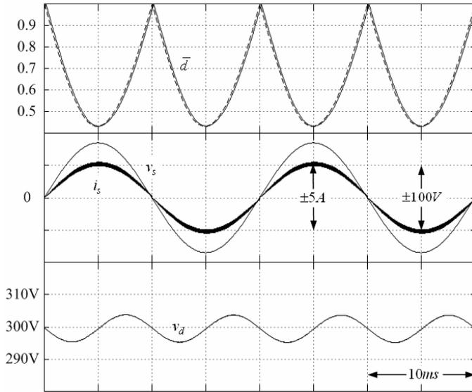
Fig. 5. Simulated waveforms for ideal circuit elements.
