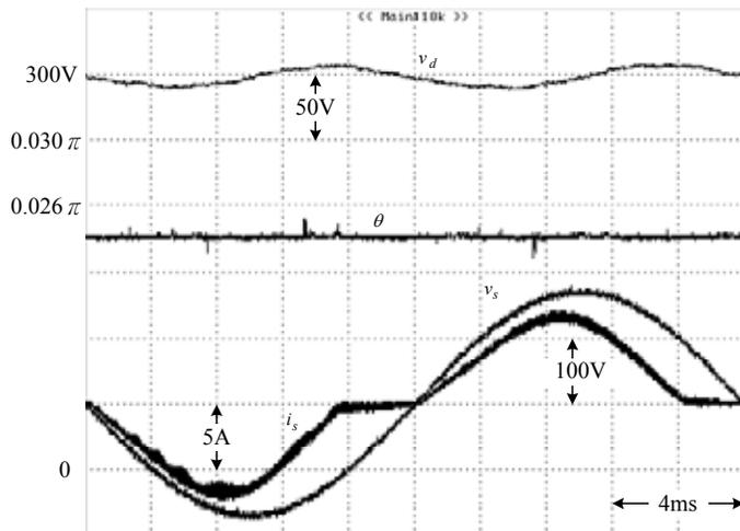
Fig. 10. Measured waveforms at  $P_s = 456W$ . Top: output voltage. Middle: duty phase. Bottom: input current and voltage.
