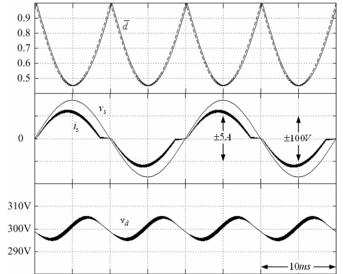
Fig. 6. Simulated waveforms for ideal circuit elements.
