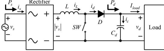
Fig. 1. Power circuit of the boost-type SMR.
