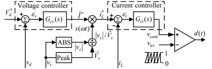
Fig. 2. Conventional multi-loop control for boost-type SMRs.
