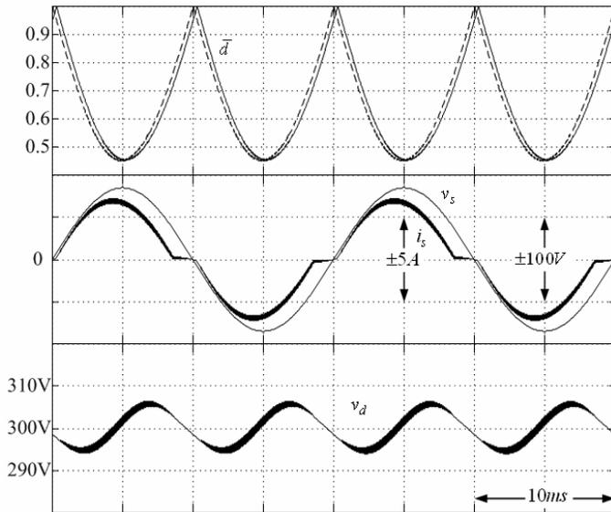
Fig. 7. Simulated waveforms for ideal circuit elements. Top: average duty signal. Middle: input current and voltage. Bottom: output voltage.
